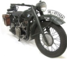
1935: R12/R17 First hydraulic telescopic fork on a motorcycle series
