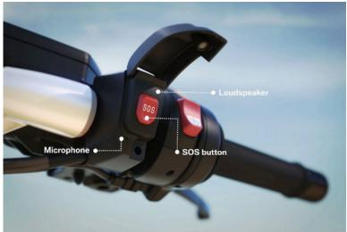
The comprehensive and intelligent sensors for accident detection enable reliable differentiation from non-accidents.
